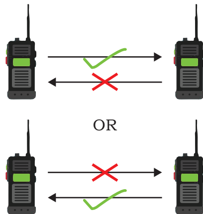
Figure 11.4: Half-duplex where communication occurs in two different moments.
